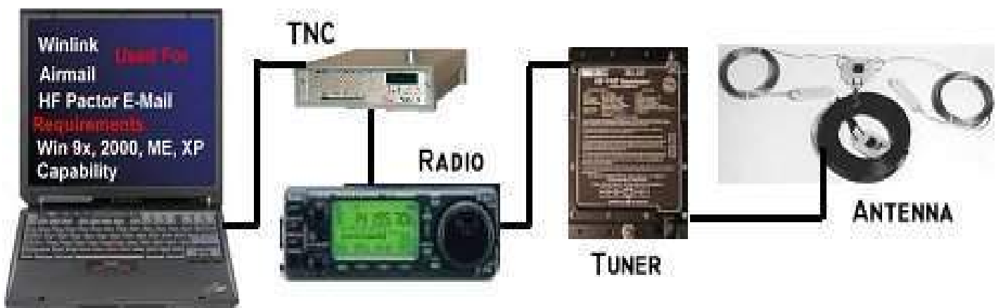
Figure 1 - Basic Equipment for HF Data/E-Mail including laptop, TNC Modem, Radio, Antenna Tuner and Antenna
